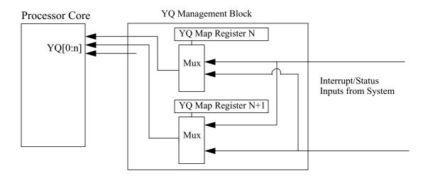
If interrupt request signals are brought into the YIELD qualifiers as described, even an interrupt condition that is masked by software so that it will not cause any exception vector to be executed can be used to enable the rescheduling of a service thread, for "zero latency" handling. On processors and VPEs using fine-grained multithreading, this
